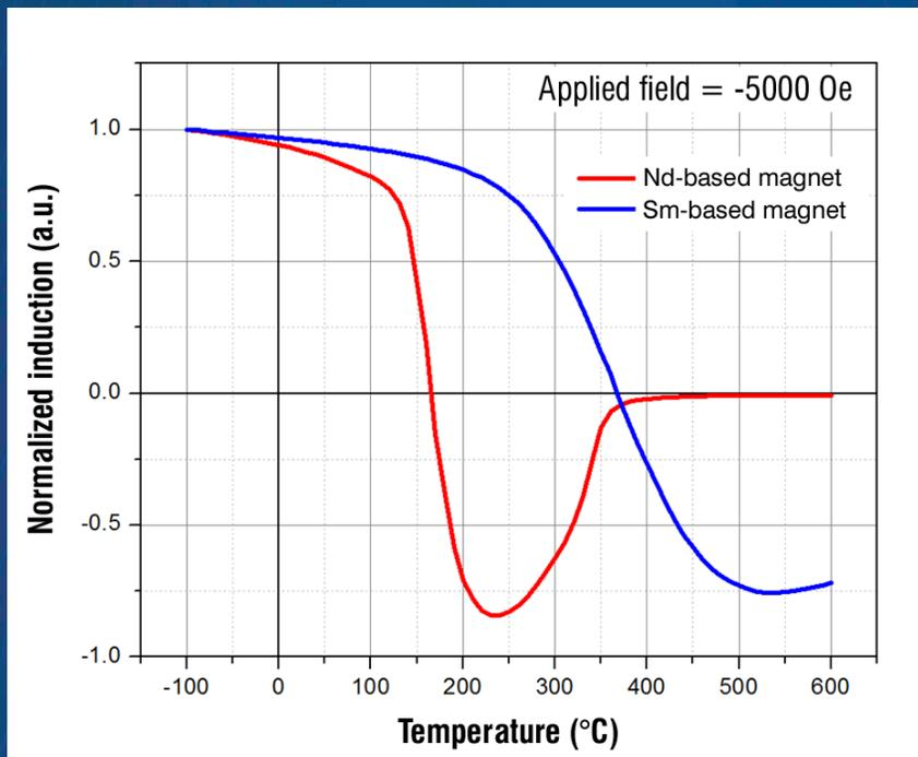
**Figure 2: Fixed applied demagnetizing field temperature dependence curves**
