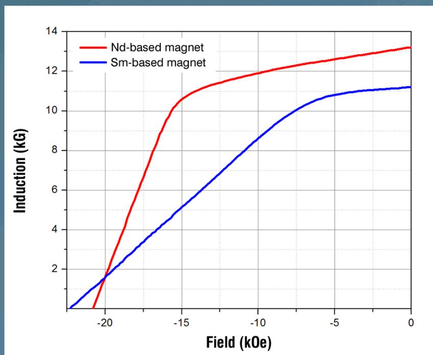
Figure 1: 2nd quadrant room temperature demagnetization curves for Nd and Sm-based magnets\*
