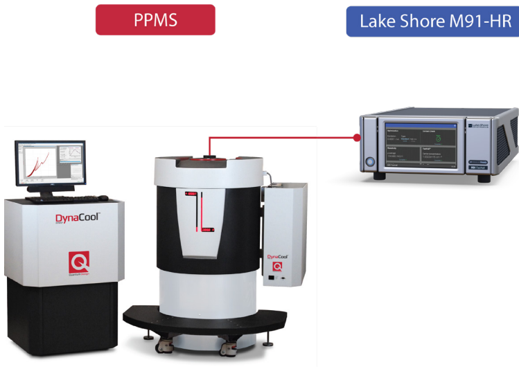
Diagram 3: PPMS connected to the M91 with the Lake Shore insert
